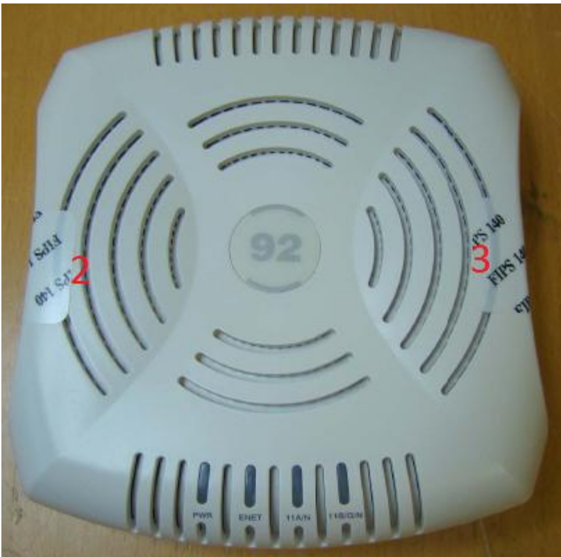
Figure 8 - Aruba AP-92 Tel placement top view
