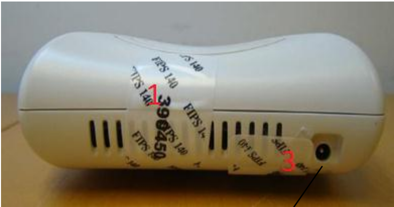
Figure 17 - Aruba AP-105 Tel placement right view
